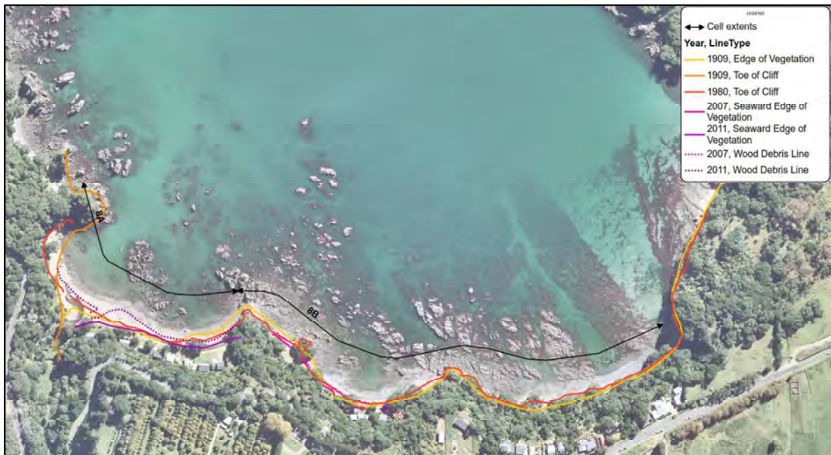
Figure 8.4: Historic shorelines along Whanarua Bay (note insufficient shoreline data was available to complete DSAS analysis)
