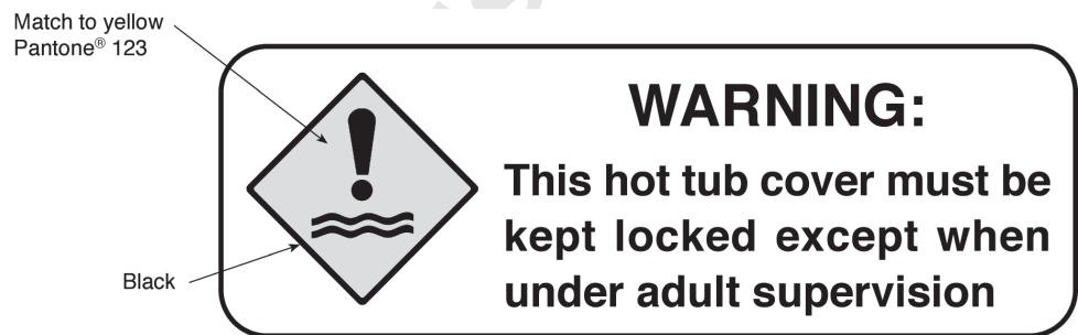
Figure G4 – Hot tub cover warning signage
