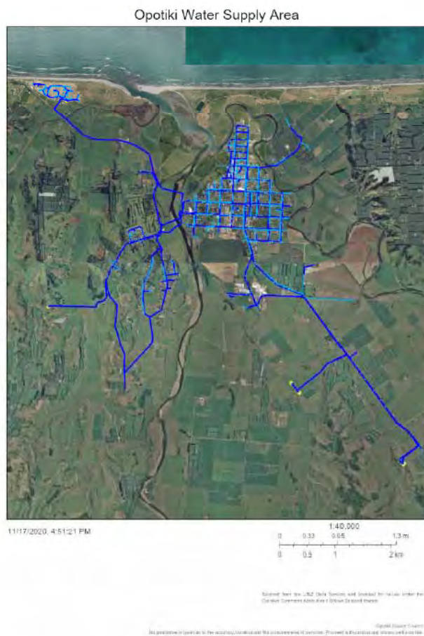
Figure 3-3: Ōpōtiki water supply network
