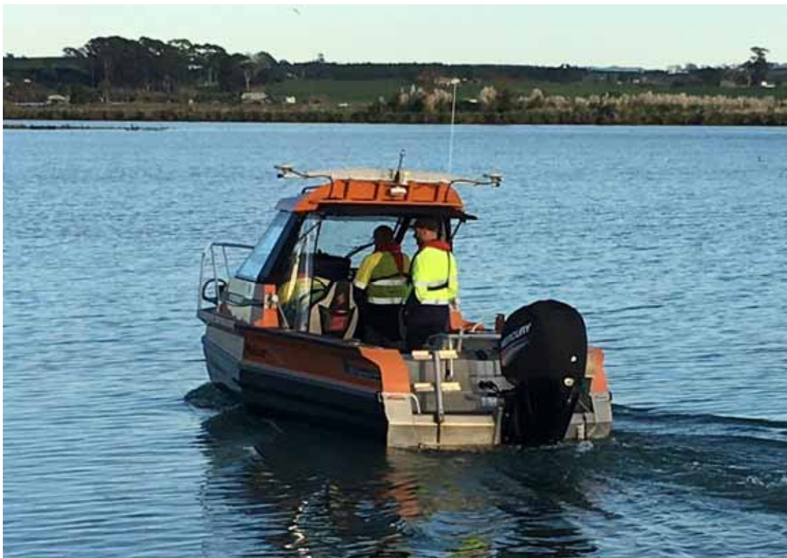
Over cover image was taken just off the Ōpōtiki wharf in May 2020 as DML began bathymetry work to get accurate depth mapping of the sea floor and river mouth area for construction planning of the harbour entrance.
