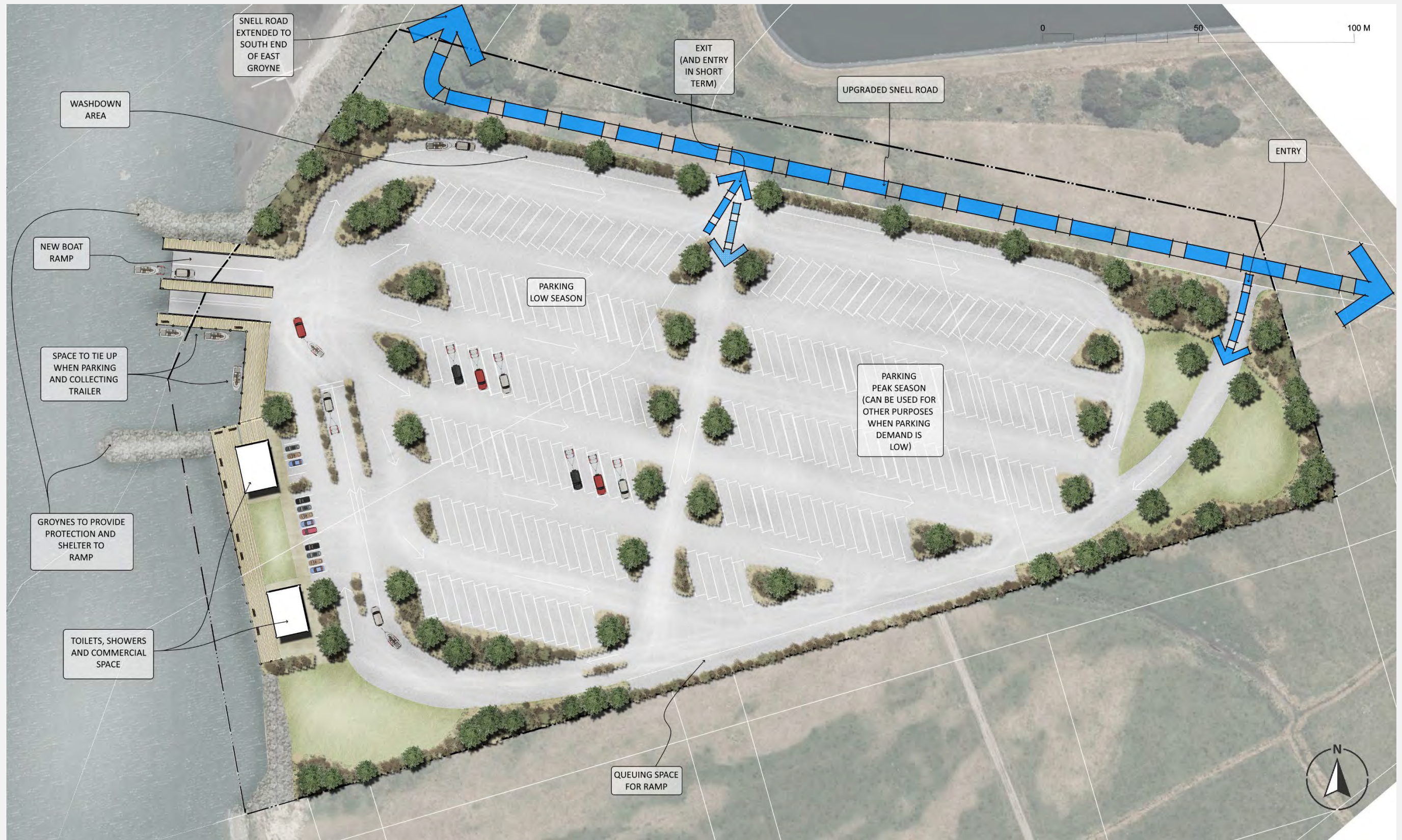
Figure 20: Masterplan layout for New Ramp and Associated Facilities, Snell Road
