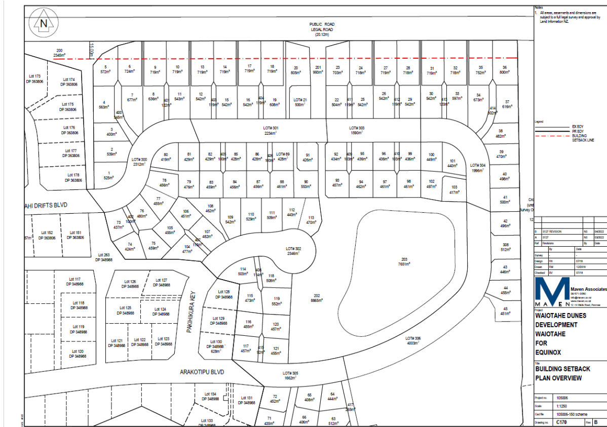
Figure 2 - Proposed scheme plan showing 15m BLR setback (for a relocatable building).
