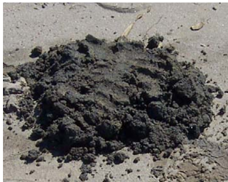
Figure 3.10 Sample 3 sand-size sediments retrieved from the eastern channel entrance, October 17, 2003. Note absence of gravel.
