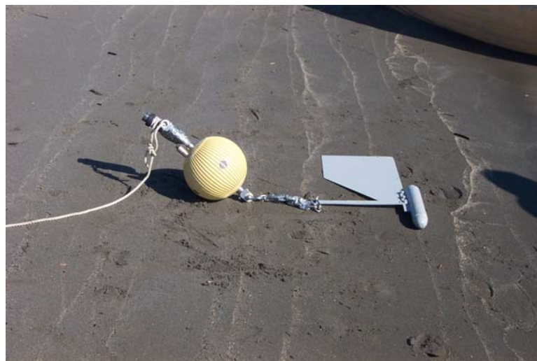
Figure 2.1 The InterOcean Systems S4 current meter and mounting system deployed in the Opotiki river entrance.
