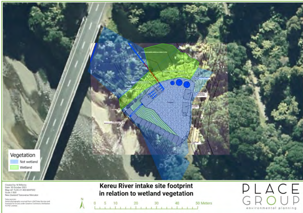
Figure 2: Works area footprint against wetland and non-wetland areas. Site plan provided by applicant.
